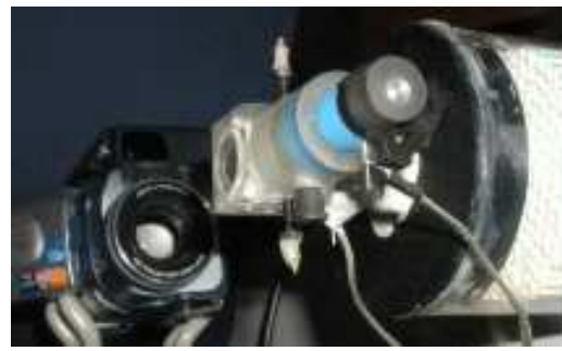
Figure 2: Video recorder to film the reed opening while the pressure blowing pressure is modified
