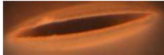
Figure 3: Sample picture of a video showing the variation of the double reed cross section at the inlet when blowing pressure is altered.
