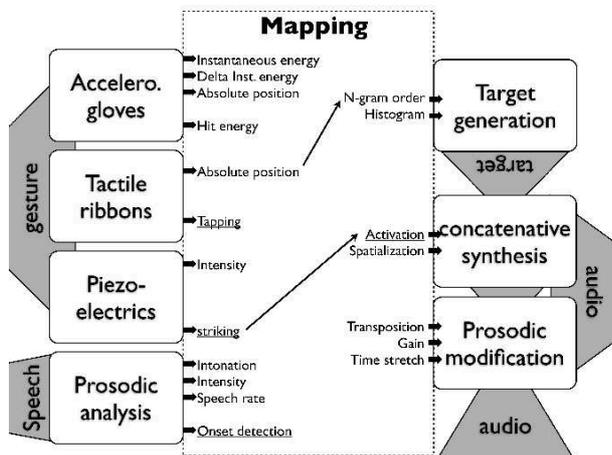
**Figure 3.** The mapping is at the interface between the data stemming from controllers (to the left) and the parameters of the audio engines (to the right). As example, two arrows were drawn. The highest allows to make vary the order of N-gram using a tactile ribbon. The lowest allows to activate a segment of the concatenative synthesis by a striking on the body.
