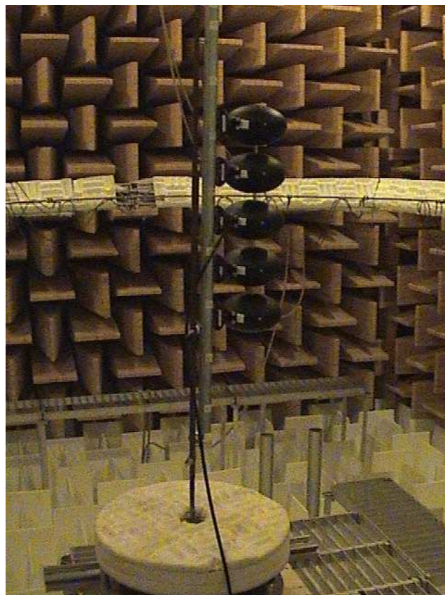
FIG. 2.14 – Measurement of an electrodynamic KEF loudspeaker mounted between four other loudspeakers (two to each side) to recreate the presence of the adjacent loudspeakers in a WFS array.
