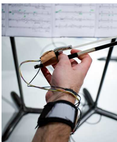
(a) The augmented violin: example of an instrumented bow
