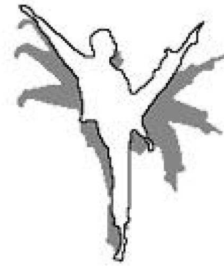
Figure 3.6: A Silhouette Motion Image with time window n=4 frames
