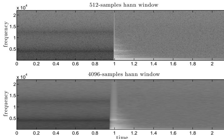
**Fig. 1.** Two different spectrograms of a B4 note played by a marimba, with Hanning windows of sizes 512 (top) and 4096 (bottom) samples.
