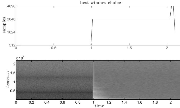
**Fig. 2.** Example of an adaptive analysis performed by our algorithm with four Hanning windows of different sizes (512, 1024, 2048 and 4096 samples) on a B4 note played by a marimba: on top, the best window chosen as a function of time; at the bottom, the adaptive spectrogram with  $\alpha = 0.7$ .
