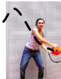
Figure 5. MO ball in with continuous control. First, choose one or several sound files and record a set of different gestures. Then, the recognition system along with the sound engine allows the user to gesturally select and control continuously parameters of the sound. For example, sound can stretch according to the pace of the gestures
