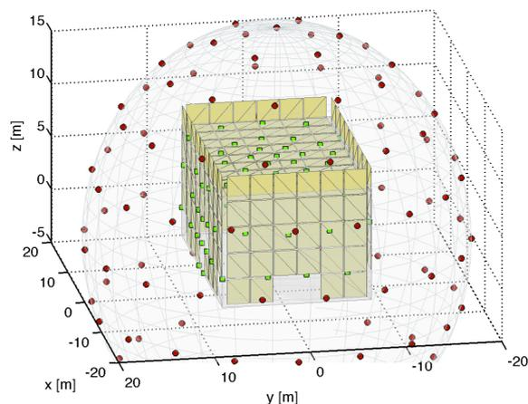
**Figure 4 – Projection of an optimal source distribution on a circumscribed sphere to the walls of ESPRO.**
