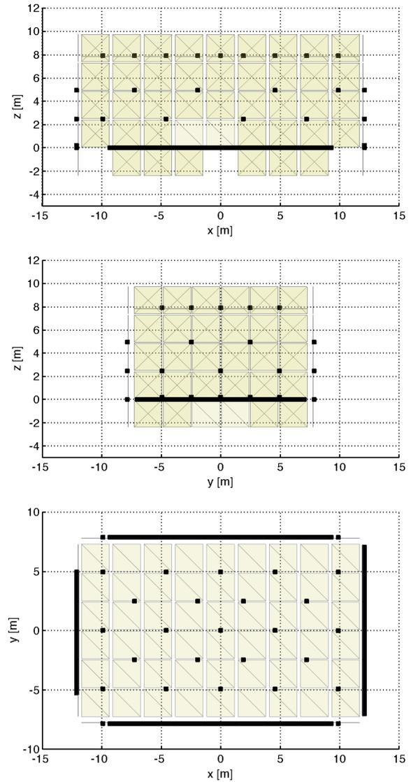
Figure 5 – 350-loudspeaker WFS/HOA array in ESPRO: vertical sections of the north wall (upper), the east wall (middle), and top view (lower)
