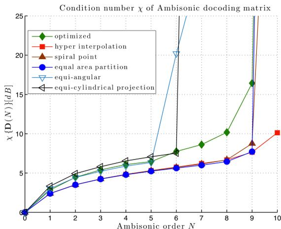
**Figure 2 – Condition number  $\chi$  of different fundamental spherical discretization schemes for a virtual set of 121 points on the sphere.**
