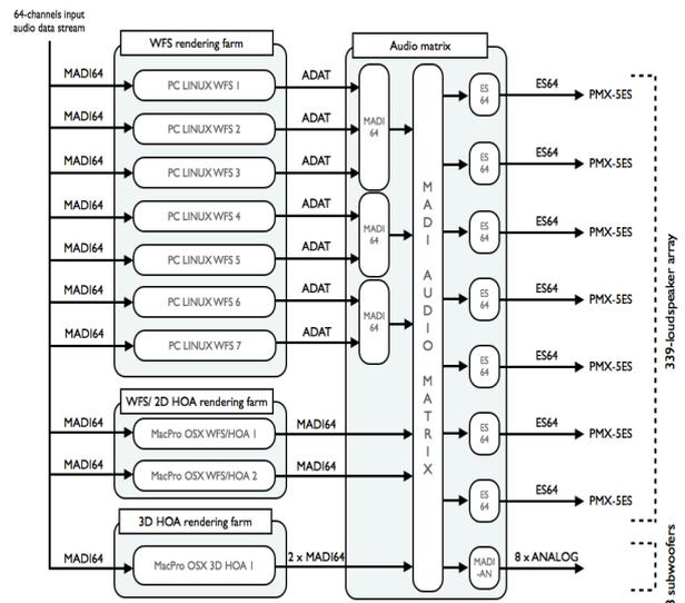
**Figure 3 – Audio processing and signal routing structure.**
