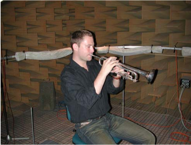
FIG. 1. Trumpet player during the directivity measurements in the anechoic chamber.
