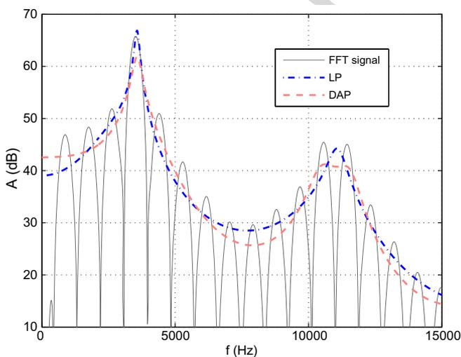
Fig. 2. LP and DAP estimations of the ARMA test spectrum (model order  $O = 25$ , sample rate  $F_s = 44,100$  Hz, fundamental period  $P_0 = 50$ ).
