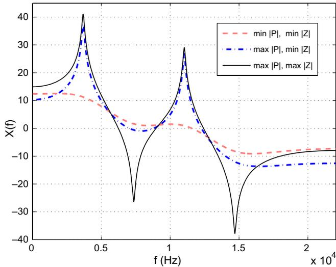
Fig. 3. Examples of the evaluation transfer functions. The solid line corresponds to a transfer function with pole/zero positions with maximal radii. The dashdotted line shows a pole dominated transfer function with maximum radii for the poles and minimum radii for the zeros, and the dashed line shows an ARMA transfer function with pole/zero positions with minimum radii.
