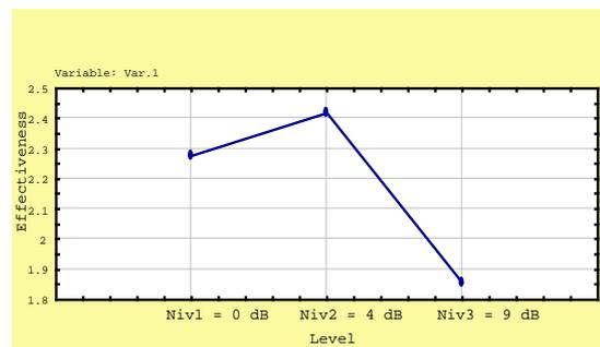
Figure 6: Effect on the effectiveness of the Level ratio between the underlining sound and the target.
