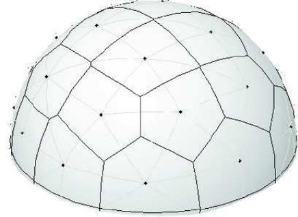
Figure 10: IEM-CUBE loudspeaker layout with Voronoi cells determining the coverage area of each loudspeaker.
